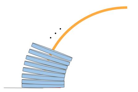
Let each disk represent a section of the continuum joint with some mass and rotational inertia.
